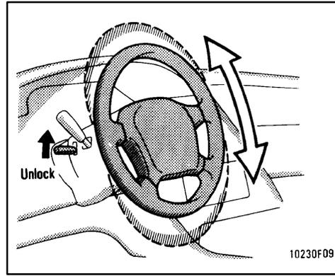
**To change the steering wheel angle, hold the steering wheel, pull up the lock release lever, tilt the steering wheel to the desired angle and release the lever.**
