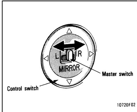
To adjust a power rear view mirror, first place the master switch at “L” (left) or “R” (right) depending on which mirror needs adjusting, then push the control switch in the desired direction.
