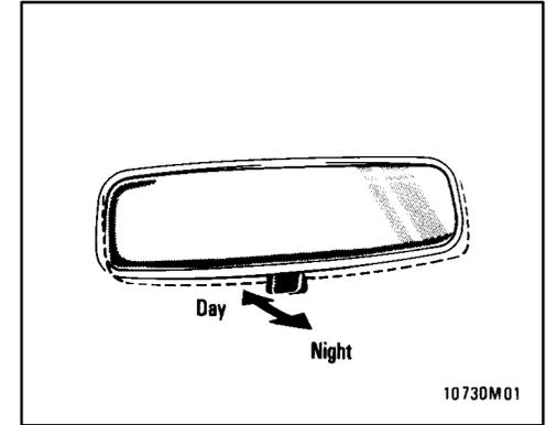
Pull the lever toward you to reduce glare from the headlights of the vehicle behind you during night driving.
