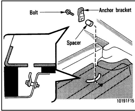
d. After installing the anchor, put the carpet back in place.
