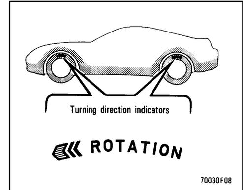
**Do not perform rotation of the tires, from front to rear or from left to right, or using the compact spare tire. Performing such tire rotation may result in the tires interfering with the body or in uneven wear of the tires, so that steerability of the vehicle is impaired.**
