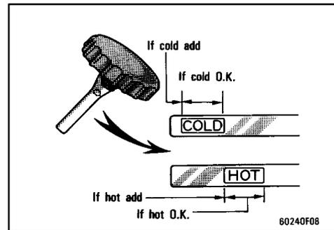
**Check the fluid level on the dipstick. If necessary, add automatic transmission fluid DEXRON® II or III.**
